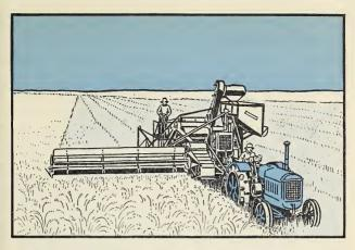
The combine first cuts the heads off the wheat. These fall on a platform and a belt carries them up into the machine. Then steel fingers, that work much faster than any man's fingers could work, knock the kernels out of the heads. Machinery pours the kernels into sacks, sews up the sacks, and drops them into wagons. It would take a great many men to do the work that one combine does.
